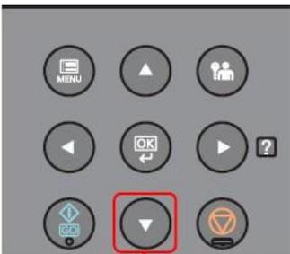
4. Press the down arrow key to show Network Name (SSID).
