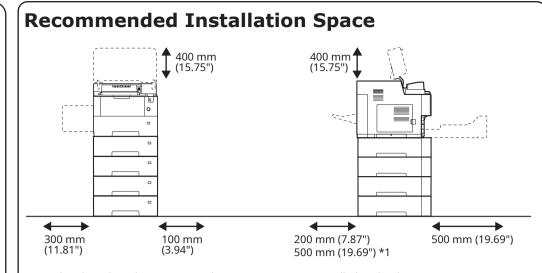
\*1: The value when an optional rear tray (PT-320) is installed to the the ECOSYS PA5000x, ECOSYS PA5500x and ECOSYS PA6000.
