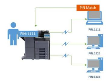
After verification, the MFP and workstation establish a HTTPS communication channel on TCP Port 19091 or higher. All further communication including image transfer occurs on this channel.
